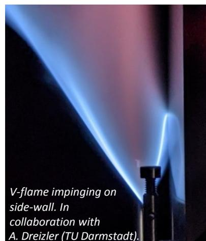
Our research utilizes a hybrid fs/ps rotational CARS approach in 1D to resolve gas temperature and species normal to surfaces. This will be coupled with LIF (OH or CH<sub>2</sub>O) to resolve flame behaviour and thermochemical states simultaneously.
